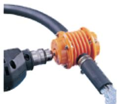
2. Affix a drill hose pump, purchased at the local hardware store, between two small diameter hoses using hose clamps. Using a large bucket
